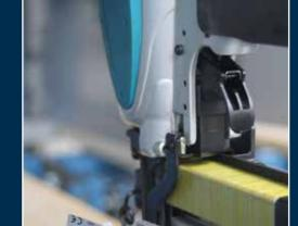
The customer's preferred make of staple gun is used. Capacity approx. 150-200 staples. Sensors warn when materials (timber, staples) are running low.
