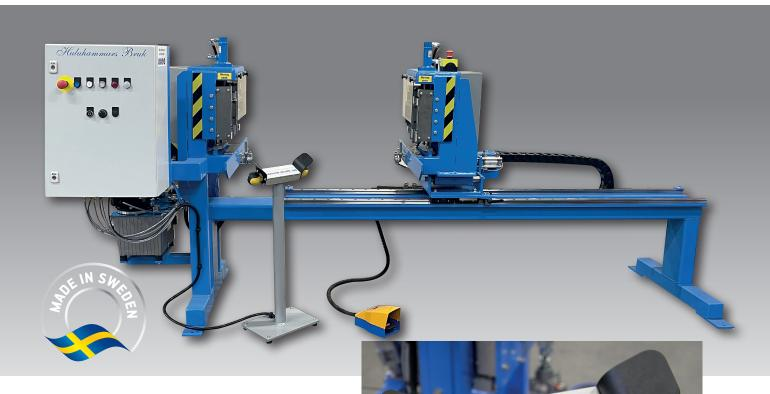
The RM Double is built on a strong machine tripod with one fixed and one moving unit on a slide for simple adjustment of material length, 543 - 2400 mm + - 5 mm, with control of material + - 5 mm for the orientation of the rivet. The rivet unit has long life heavy duty bearings for the spindle. The rivet design is adjustable between 3 - 10 sec.
